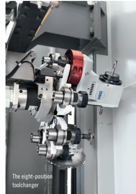
"If you have a particular fitting such as a Clamex, you can use the saw blade for this."
