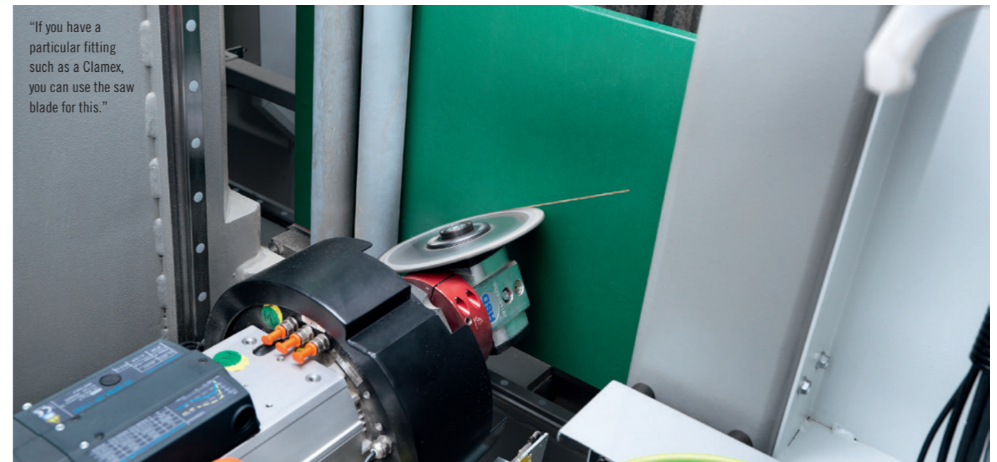
The eight-position toolchanger
